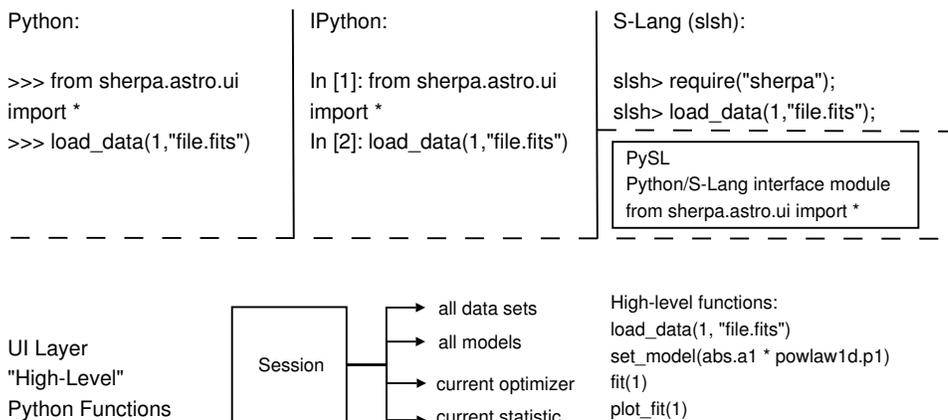
Figure 2. *Sherpa* modules in a variety of environments.
