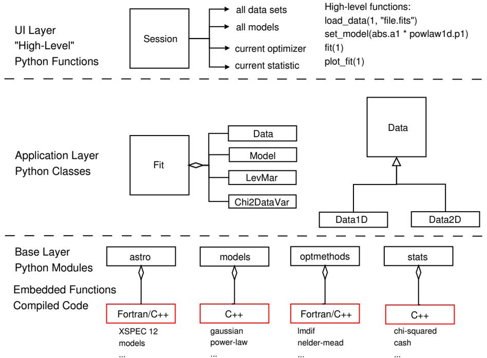
Figure 1. Base, application, and UI layers of the *Sherpa* design.
