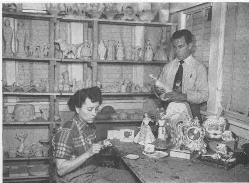
THE CERAMICS WORKSHOP of Yetta and Cecil Garringer is a storehouse of fine art work. The shelves hold the clay "greenware" as it comes from the mold. On the table are some of the finished products. The lineup of clocks shows them in the mold, greenware, bisque and final form.
