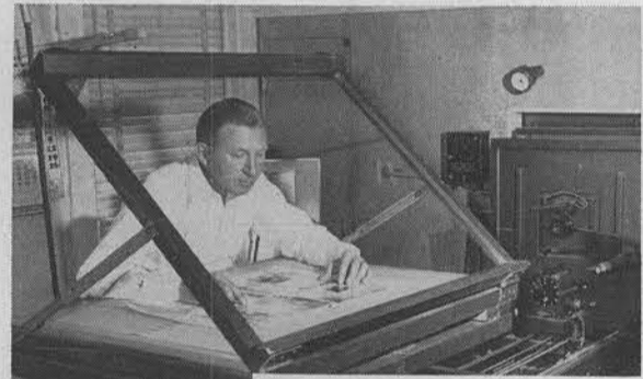
SKILLED CRAFTSMEN at the same time are working on zinc halftones at the engraving plant. A photographic process involving light-sensitive metal plates results in clear, sharp pictures in the finished paper.
