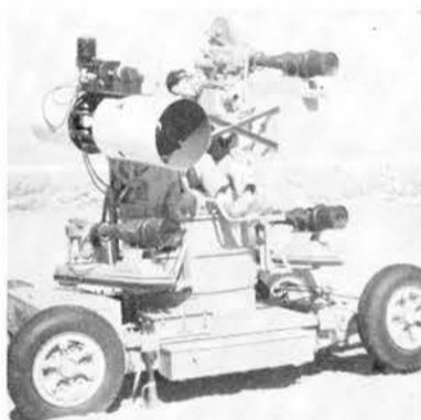
ANTI-AIRCRAFT GUN MOUNT is used to support a battery of high-speed movie cameras which track the path of falling "dummy" bombs at Yucca Flat.
