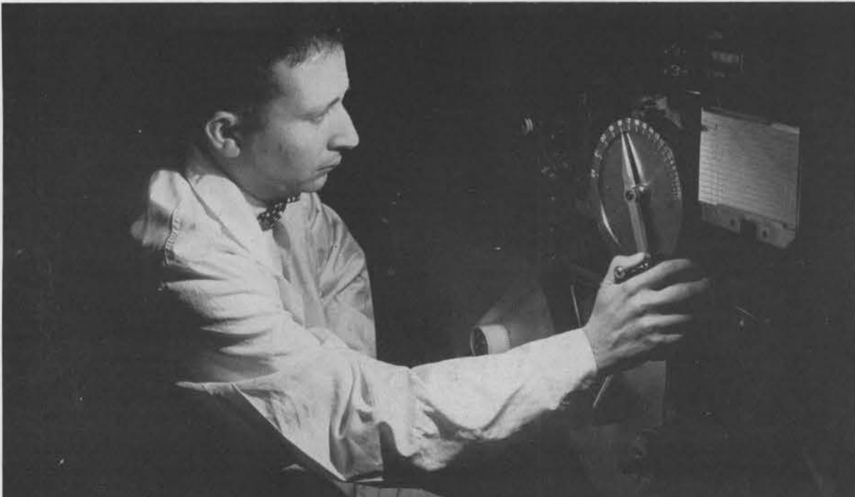
DUPLICATING the original print after editing, Skip Baca adjusts the exposure control on the printing machine. Since the original film had variations in exposure, the duplicate print has to receive the same exposure or corrected exposure. With the printer, it is possible for Skip to change color density and tone. Both the exposed film and the raw film move through the printer at the same time.
