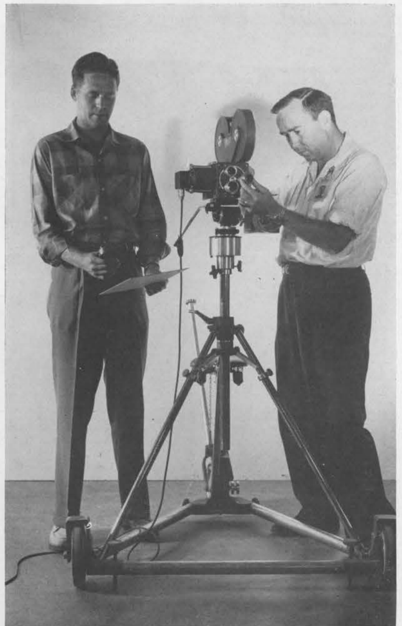
LIGHT EXPOSURE is read by Wayne Hancock, left, as Bob Matthews sets the reading on the movie camera. The Motion Picture Division's studio in Bldg. 808 is equipped with floodlights, overhead spotlights and auxiliary lights. The camera rests on a wheeled dolly that allows smooth following of moving subjects.
