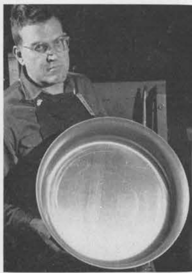
FINISHED PRODUCT is this aluminum "bowl" formed from a disk of the ductile metal.
