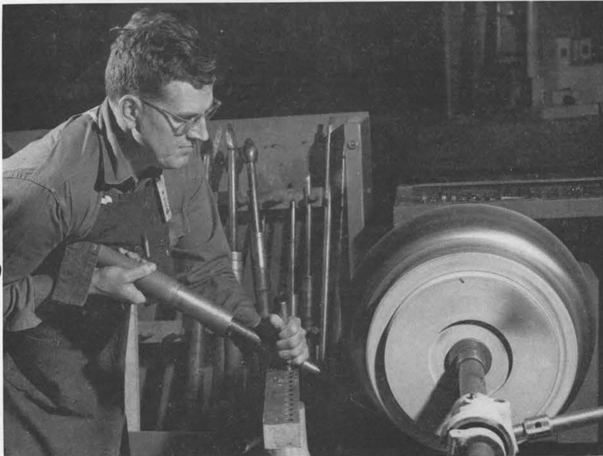
SPINNING ALUMINUM is accomplished by Burrell Snelling (2151) who bends aluminum disk over wooden form as it revolves on a lathe. Pressure on the spinning tool Burrell is holding shapes metal.
