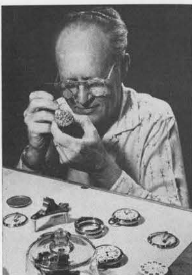
DELICATE MODIFICATION to a commercial railway watch is performed here by Everett Click. Using this mechanism for the heart of a precision escapement timer reduces considerably the cost of special Sandia prototype.
