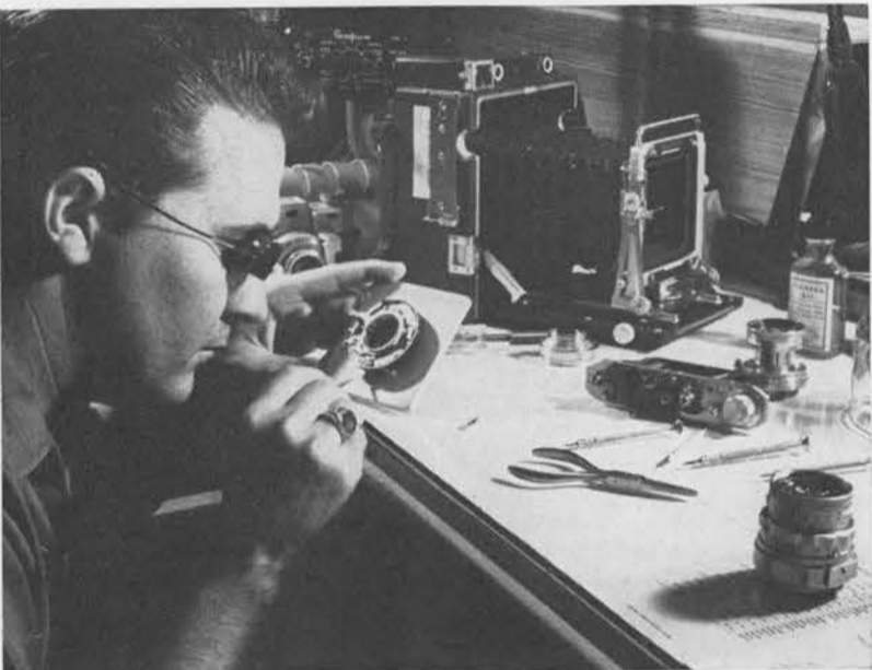
INSTRUMENT REPAIRMAN W. C. McGrew, a trained watchmaker, is shown here adjusting the shutter mechanism of a press camera sent to Section 4231-3 from the photographic laboratory.
