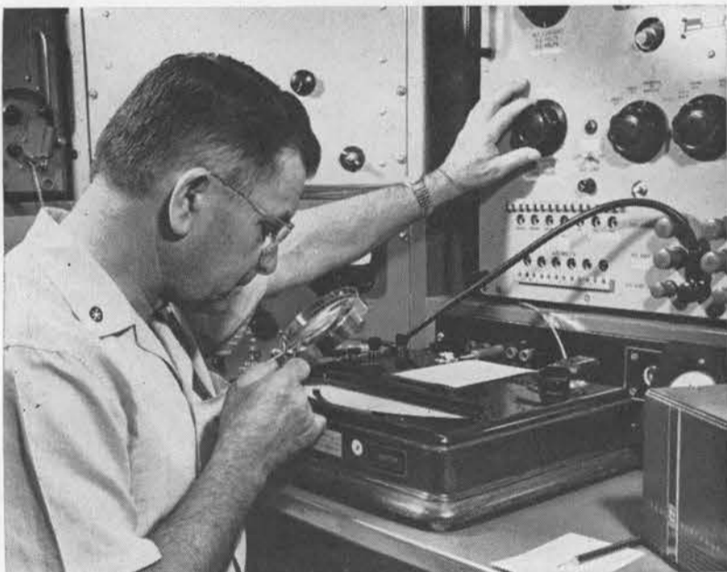
ACCURATE READING from a precision millimeter is taken by Charles Skaloud who uses a magnifying glass to insure a precision adjustment. Section calibrates all instruments repaired in the shop.
