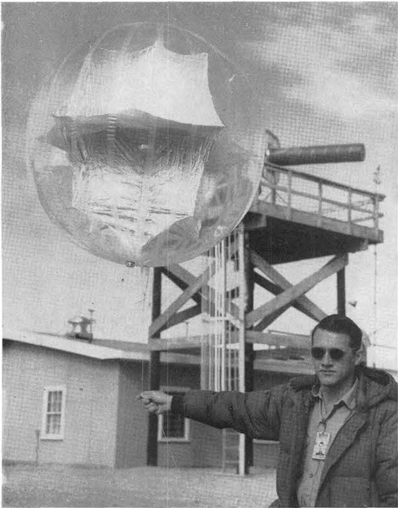
MYLAR BALLOON with aluminized reflector inside which can be detected by radar is held by Charles T. Force (7131-2) at Tonopah Test Range. Balloon is of type to be used at Point Arguello, Calif., for measuring high altitude wind direction and velocity.
