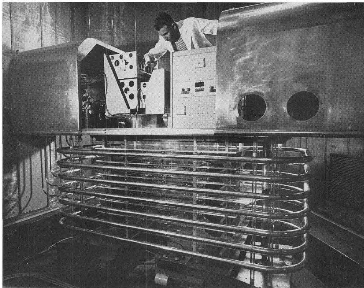
HIGH VOLTAGE STACK of Cockcroft-Walton accelerator is contained in temperature and humidity controlled room. Aluminum domes on either side of R. I. Ewing (5150) close during operation.
