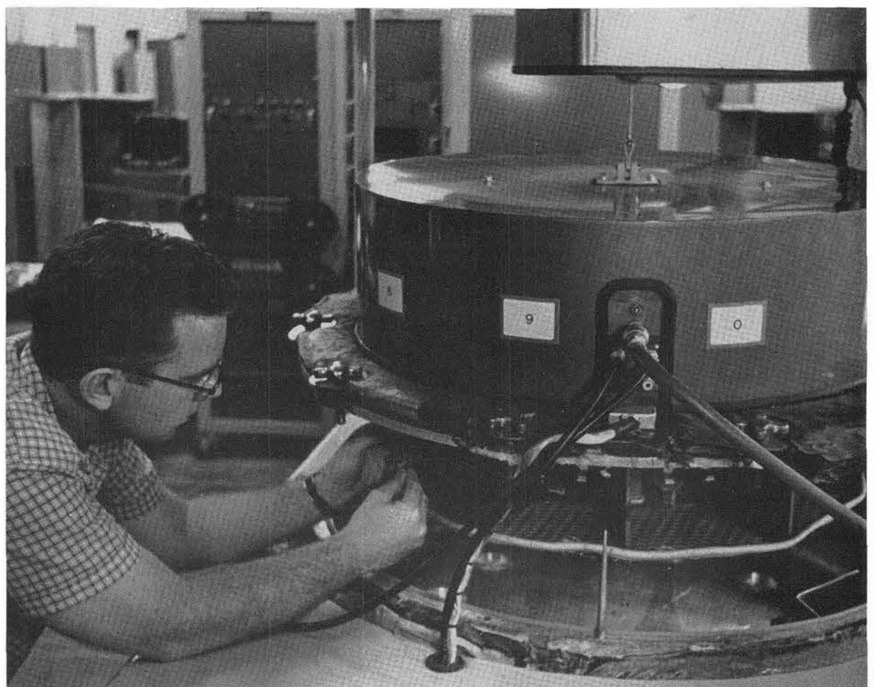
REVOLVING TEST HEAD of the APAR tester in use in the Environmental Test Operations Department laboratory accepts up to 10 small Krypton
