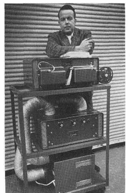
BABY APAR tester is displayed by George H. Donaldson (2452-2). Utilizing same principles of automatic programming and recording as full-size APAR, the junior machine was developed as a mobile laboratory instrument for automatic testing of components in Sandia advanced development organizations.
