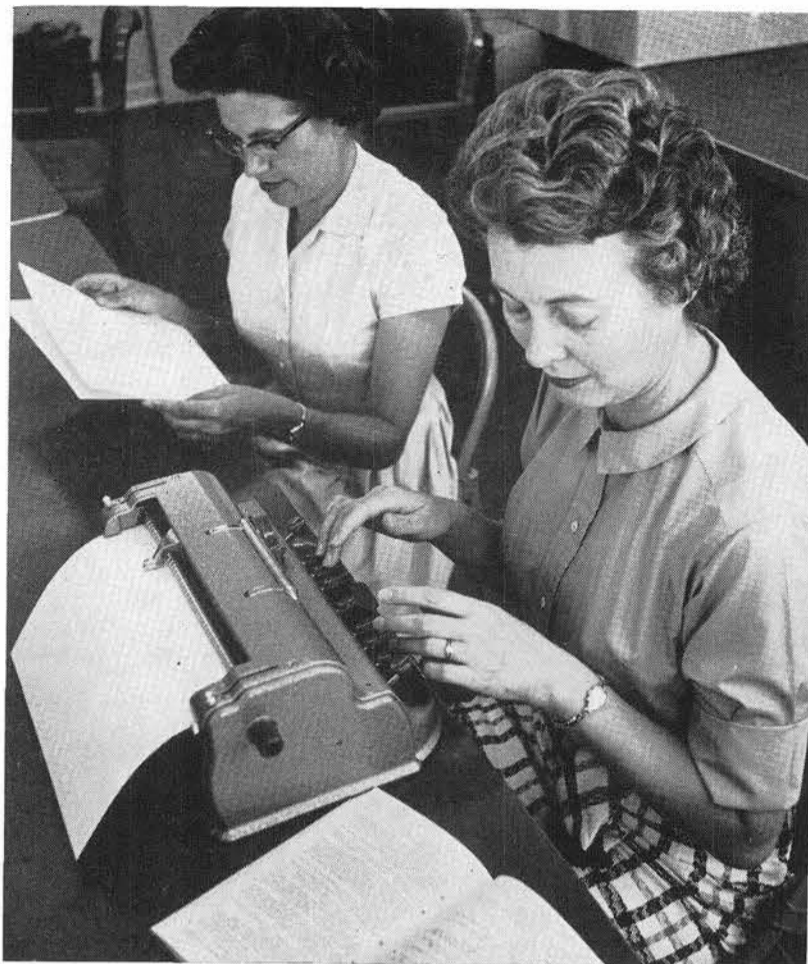
SIX-KEY BRAILLING MACHINE, which punches raised dots in paper, is used by Evys Warren (1442) to transcribe English into the language of the blind. Different dot combinations form all 26 letters of the alphabet. At right, Elizabeth Frost (1442), also a Brailist, checks copy which Evys has just typed.
