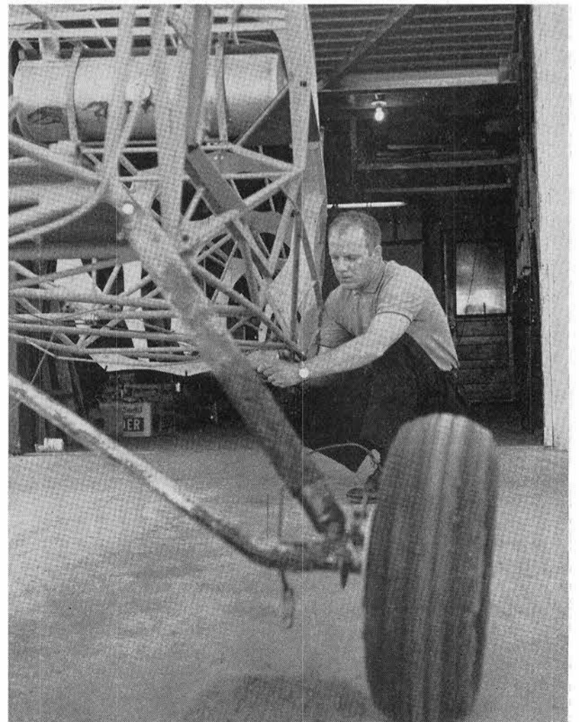
CURRENT PROJECT in Bill Guernsey's garage workshop is the total renovation of a 1941 Aeronca "Chief." Framework was completely disassembled and rebuilt with new parts made by using the old ones as patterns. Some of the metal structure was salvaged.
