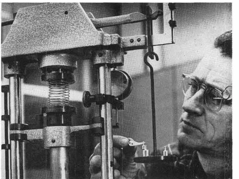
AMOUNT OF FORCE in a spring is measured by R. G. Brooks (4232-4). Total weights indicate spring force for given length.
