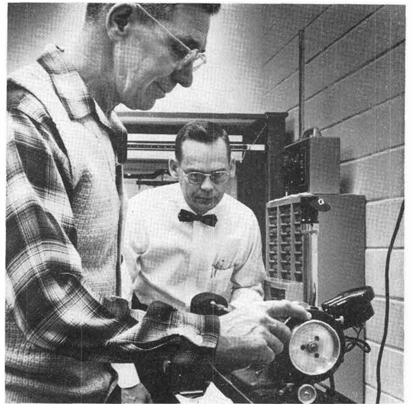
LENGTH MEASUREMENT , with direct readout to .000010 of an inch, is possible with this device in Mechanical Standards Section 4232-4. Machine, being operated by E. A. Kraehling, will measure items up to 80 in. Supervisor H. M. Meidal (right) awaits results.
