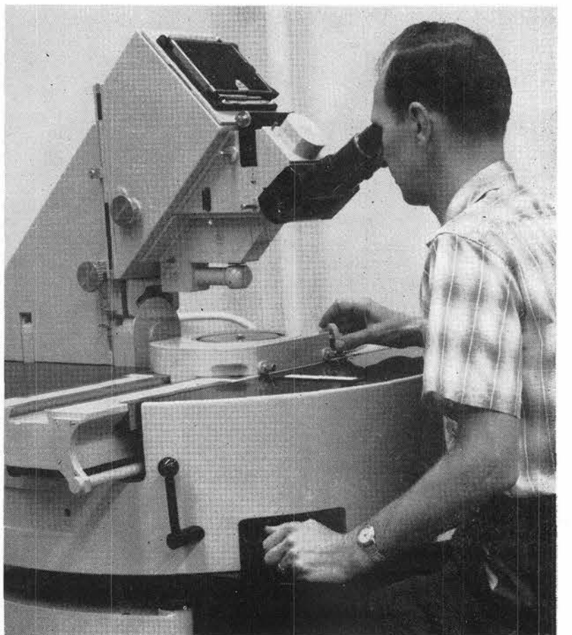
UNIVERSAL MEASURING MICROSCOPE operated by E. T. Bureta (4232-4) is being used to evaluate a small gaging device.
