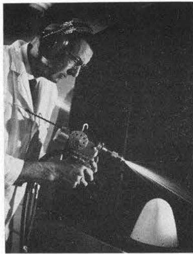
HOT spray of ceramic material is prepared for application to nose cone by Vernon Arnold (1124-1) in coating and surface chemistry lab. Headset shuts out excessive noise of operation.
