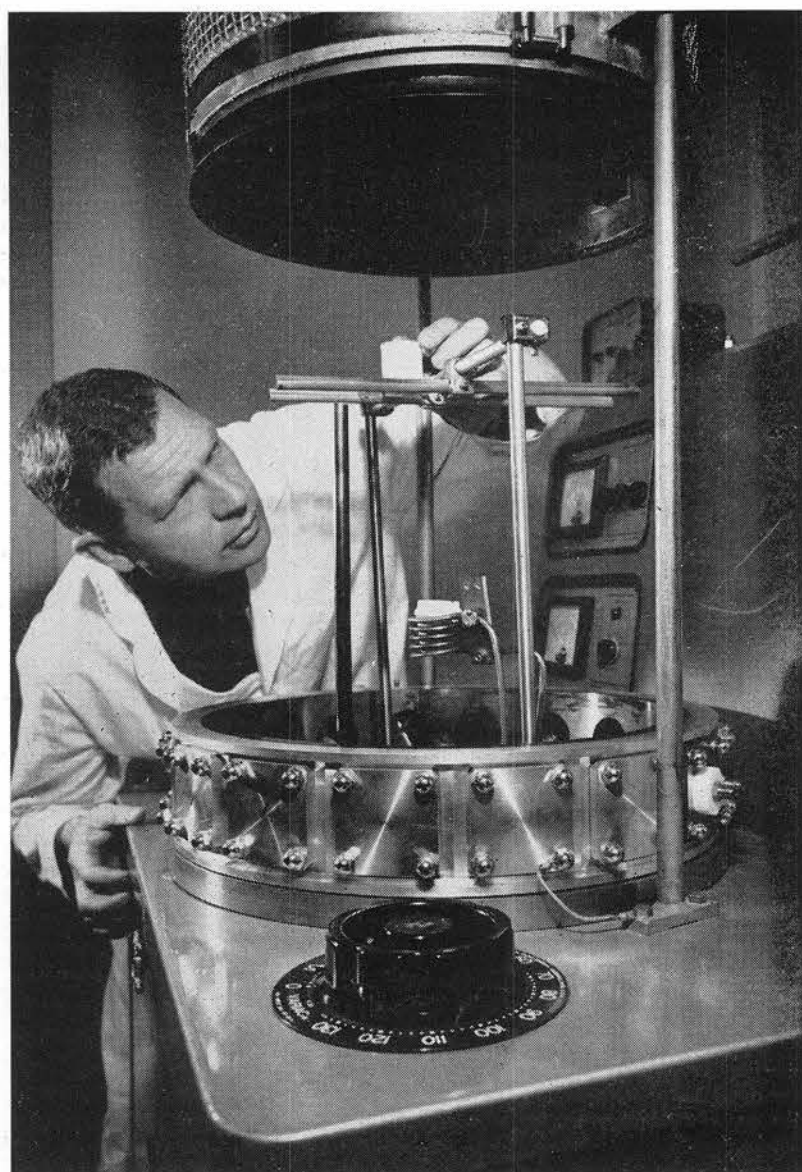
MATERIALS & PROCESS DEVELOPMENT —This issue of the Sandia Lab News contains the story of Organization 1100. Symbolic of 1100 work, Technical Staff Member Harry R. Holmes inspects material to be metal coated in a vacuum metalizer. The story of Organization 1100 starts at the bottom of this page.
