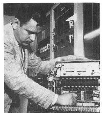
FLEXOWRITER READOUT , part of an APAR, automatic testing machine, is repaired here by Phil Archuleta.
