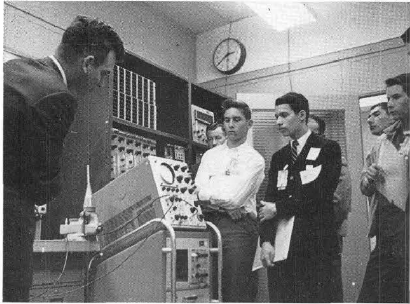
TRANSMITTING INFORMATION from missiles in flight is explained by S. G. Cain (8122-3), as CSF students see how a physical force can be converted to an electrical impulse and read out on an oscilloscope. Temperature, pressure, and vibration were shown.
