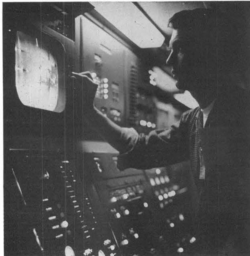
INSIDE RADAR TRAILER, Robert Germain tunes in television which is focused with a telescope lens at object radar antenna is tracking.
