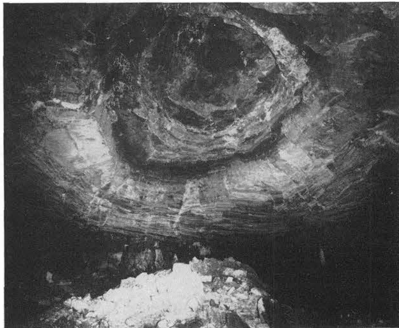
LOOKING UPWARD from the floor of the Gnome cavity, one sees stalactites. The cavity is larger in diameter than the base of the dome of the U. S. Capitol building. The cavity was created Dec. 10, 1961, by a three-kiloton nuclear detonation — the first experiment for peaceful purposes.
