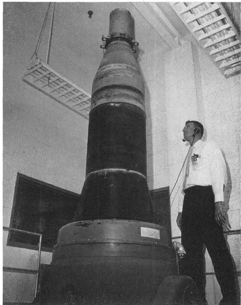
RE-ENTRY VEHICLE, designed by Sandia Corporation for use in the aerospace nuclear safety program, is shown being subjected to a development vibration test at Sandia Laboratory. At right, Denny L. Krenz (7331) observes the vehicle as James A. Enlow (7324) relays information from the control console in another room. A mockup of the core vessel for the space-bound reactor is shown on top of the vehicle.
