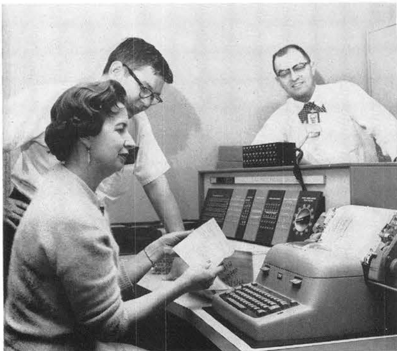
ADAPTATION OF SHAPE PROGRAM to automatically compute weight, center of gravity, and moments of inertia of a proposed component is checked over by computer operator Ann Crow, and mathematicians Freddy Whitworth and Herb Turnbull (all 8142-1). IBM 1620 Computer is used in numerical description programming for SHAPE (Sandia Hi-Precision Automated Parts Engineering), and for SPEED (Sandia Program for Engineering Etched Designs). The programs control milling machines.
