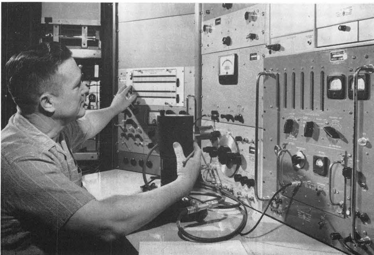
CALIBRATION TECHNIQUE, using frequency derived from crystal oscillators in AC and RF Standards Section 2412-1 laboratory, is demonstrated by J. B. Gibbons. The instrument resting on table is frequency meter.
