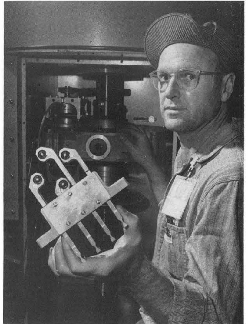
THIS GAUGE is used to determine the friction adjustment between three discs in a centrifuge. Henry R. Welch (4512) worked to manufacturer's specifications in fabricating this tool at Sandia Laboratory.
