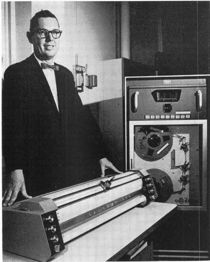
AUTHOR of a continuing program enabling IBM 7090 Computer to print with upper and lower case letters, italics, and special punctuation marks is D. K. Robbins, supervisor of Consultants and Training Division 7624. Calcomp Plotter draws letters from signals on magnetic tape.
