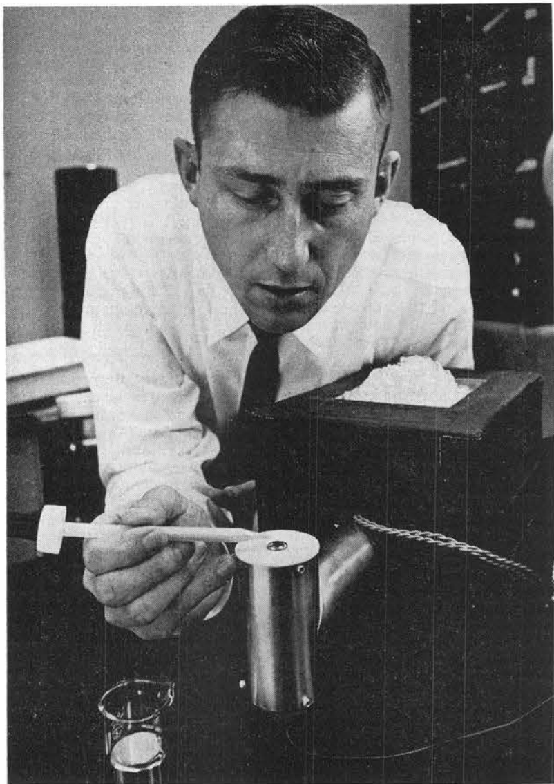
POOL OF MERCURY is placed over surface of thermocouple in a new hygrometer developed by John L. Hartley of Environmental Standards Division 2411-2. Thermocouple makes accurate dew-point measurements from moisture formed on surface of the small pool of mercury.
