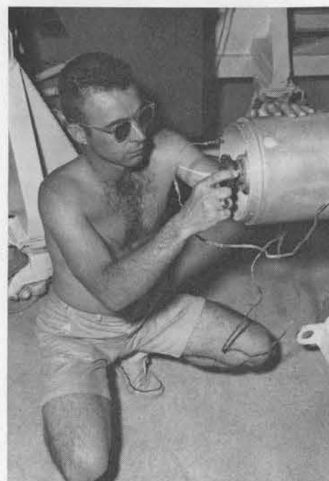
LES LUEHRING places an ignitor into a Tomahawk rocket. The operation is one of the final acts before rocket is assembled and placed on launching pad for firing. Les is in Carrier Development Division, Upper Atmosphere Projects Department.
