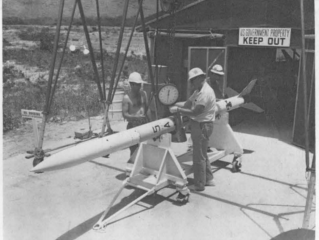
TOMAHAWK second stage rocket and nose cone containing an instrumentation package are weighed prior to placement on the launcher. Performing the operations are, from left, Les Luehring, Clem Sproul, and Jim Stracina, all of Carrier Development Division, Upper Atmosphere Project Department. All photos were taken by Holmes and Narver, Inc., photographers Barney Hatfield and Bill Telaak.
