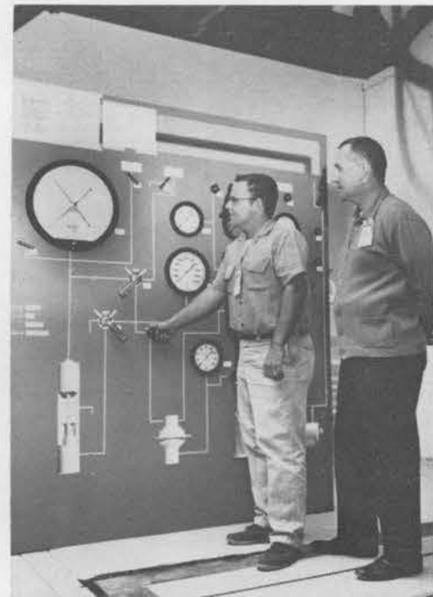
THIS HYDROSTATIC TEST CONTROL PANEL regulates liquid pressure used to hydro-test a specimen. Shown at the controls are Jim Duggar (left) and Joe Sladky, supervisor of Area 8 Environmental Test Section.
