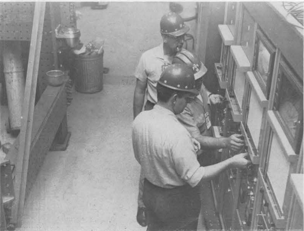
CONTROLS FOR THE STATIC TEST FRAME are set by (front to back) Bill Purcell, Jim Duggar, and Phil Sites. Static tension and compression loads are applied to a test specimen for checking the structural integrity of the part or component.
