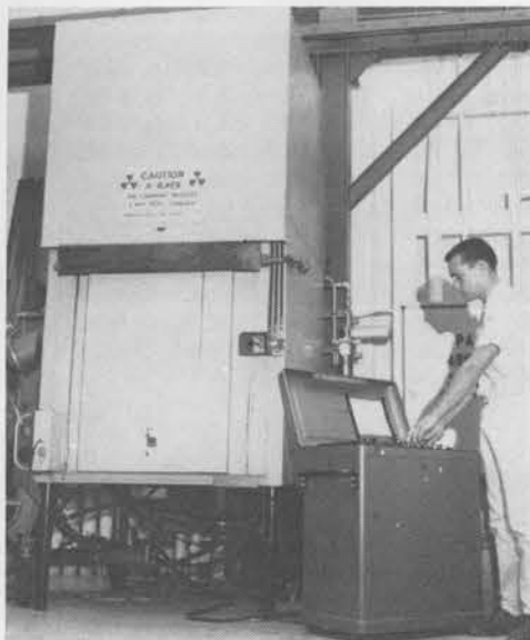
X-RAY FOR CHECKING COMPONENTS. Bob Eastburn operates this 150/300 KVA x-ray located in the hazardous test facility, Building 972. After a specimen is subjected to a test, the x-ray is used to detect cracks or other malformations resulting from the test.
