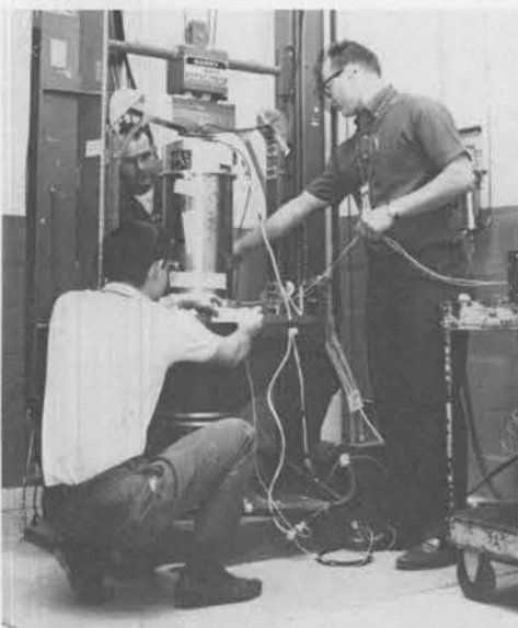
AN INSTRUMENTED TEST on the drop table is prepared by (l to r) Dennis Meyers, Les Jones, and Duane Sillanpaa. The drop table can lift a test specimen weighing up to 200 lbs. as high as eight ft., then release it to fall unrestricted, striking the anvil (table). Contact material on the table can be varied to produce the desired shock load on the specimen.
