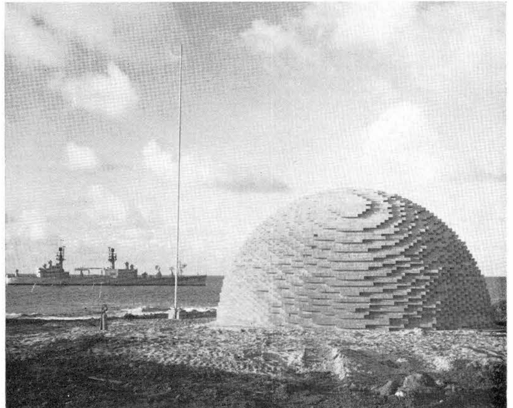
500 TONS OF TNT were stacked in this configuration before being detonated on the island of Kahoolawe this month. Three Sandians were on the ship anchored 2000 ft. from the blast.
