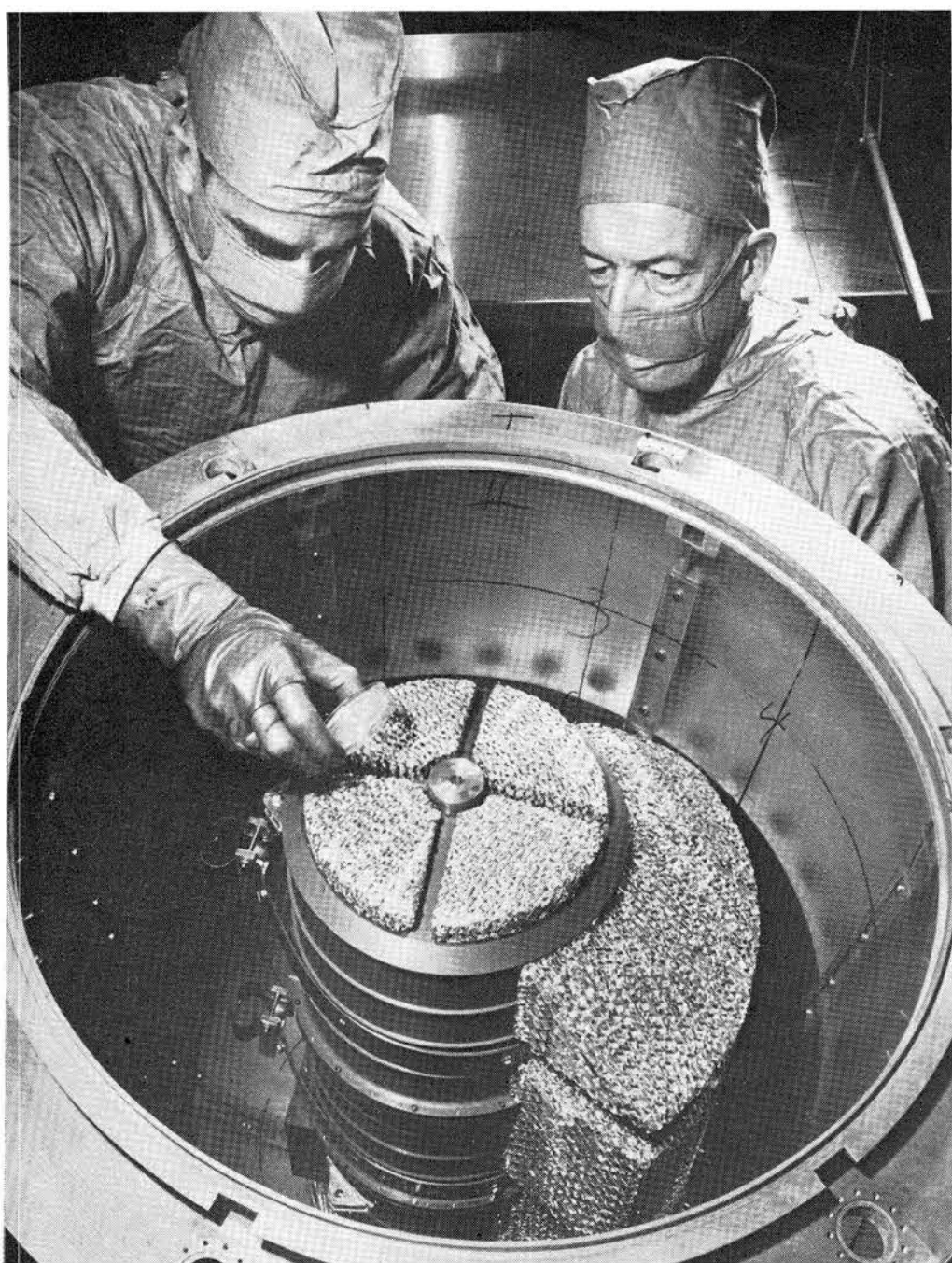
SURFACE CONTAMINATION of the space craft is checked by NASA's Ed Powers who presses a Rodac plate directly onto the cushioning material of the vehicle. The plate is incubated and the bacteria colonies, if any, which form are counted. Sandia's Vernon Arnold, right, assists in the study.
