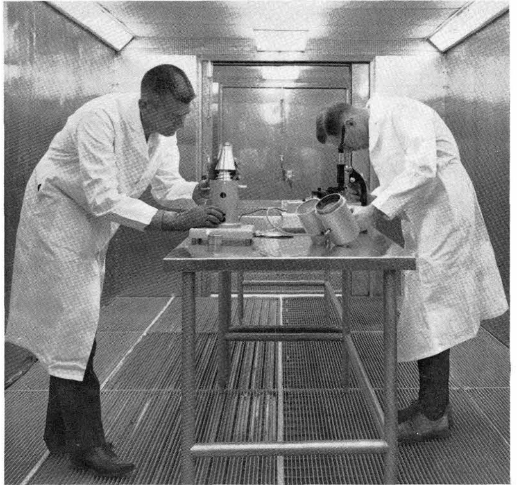
BIOLOGICAL CONTAMINATION STUDY conducted in Sandia's laminar flow clean room shows that the room's ability to control airborne contamination approaches a sterile environment. William E. Neitzel, left, and Claude Marsh of Advanced Manufacturing Development Division prepare air sampling devices used in the study.
