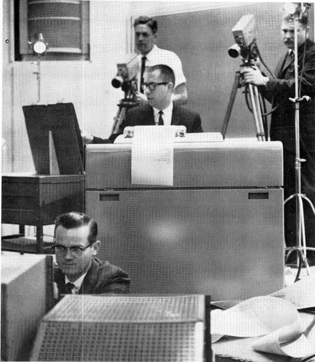
TOM FOX at Teletype keyboard demonstrates a "Compatible Time-Sharing System" for rapid man-machine interaction. The keyboard was connected directly with a computer at Massachusetts Institute of Technology via the AT&T TWX network. Howard Hayden, foreground, operates video recorder while Wayne Hancock and Elliot Harris operate TV cameras.
