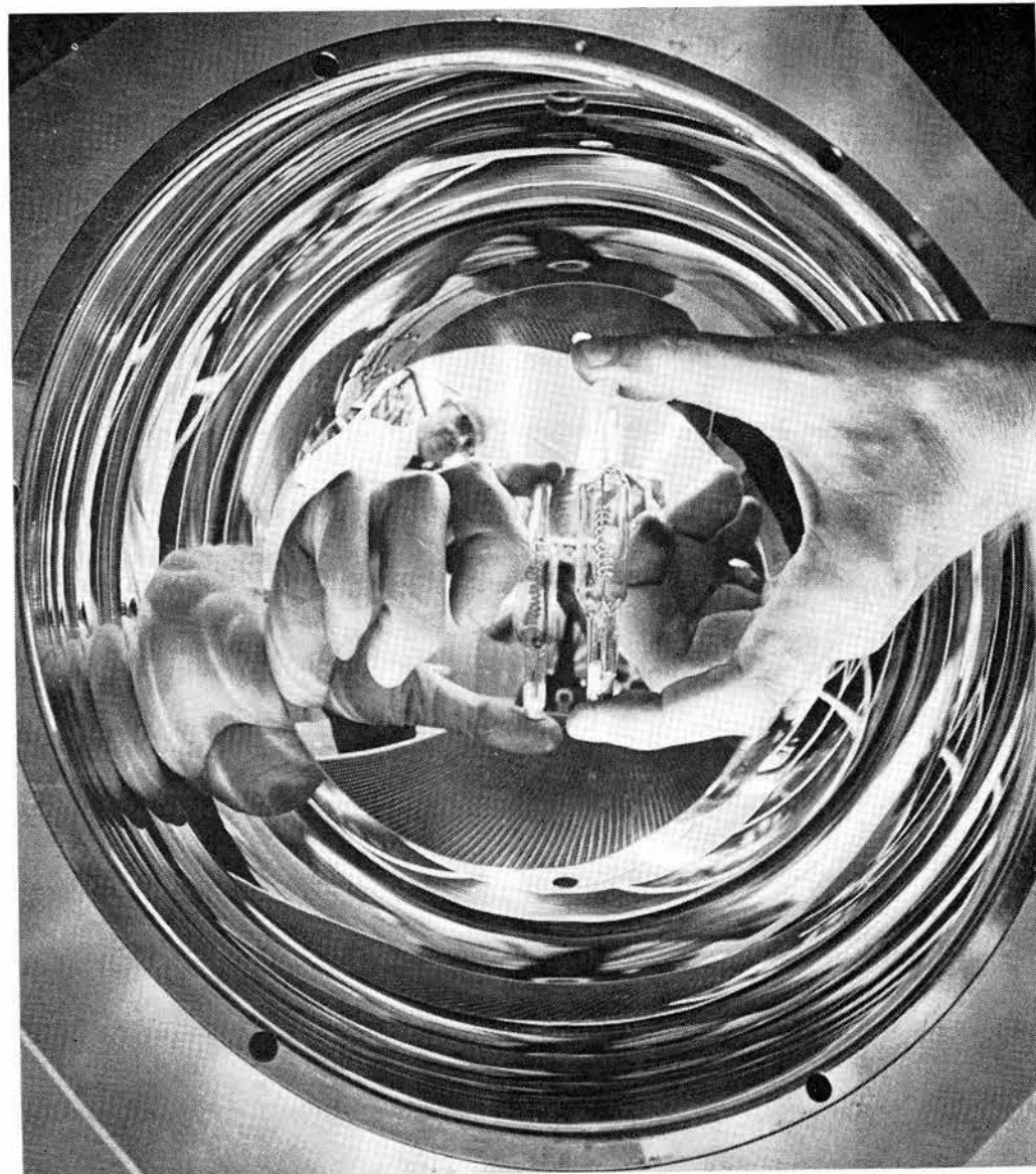
QUARTZ IODINE LAMP which powers the infrared heater is the same type unit used in home movie lighting. Photo shows some of the weird optical effects produced by the gold-plated elliptical spheroidal reflector.
