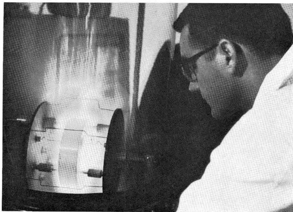
R. D. BLAND (1123) observes the ion bombardment cleaning of a SPR fuel ring. All radioactive materials are contained within the glass bell jar. Sandia has coated the uranium fuel of SPR with a thin film of aluminum, a unique achievement.
