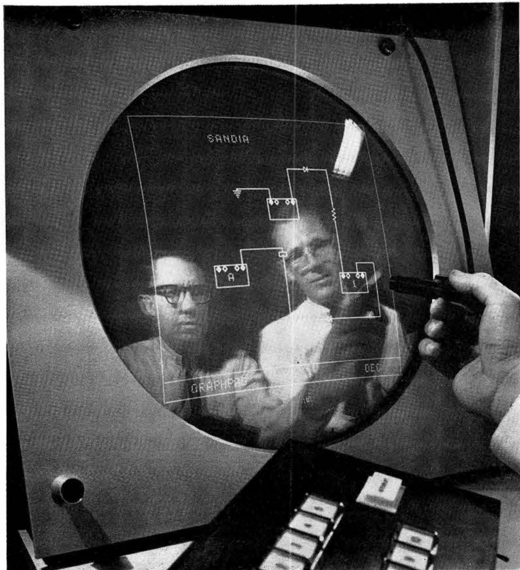
USING A LIGHT PEN to sketch an electrical circuit as part of a demonstration program on the new Sandia computer graphics system are B. T. Fox (9427), left, and C. R. Martell (2223).
