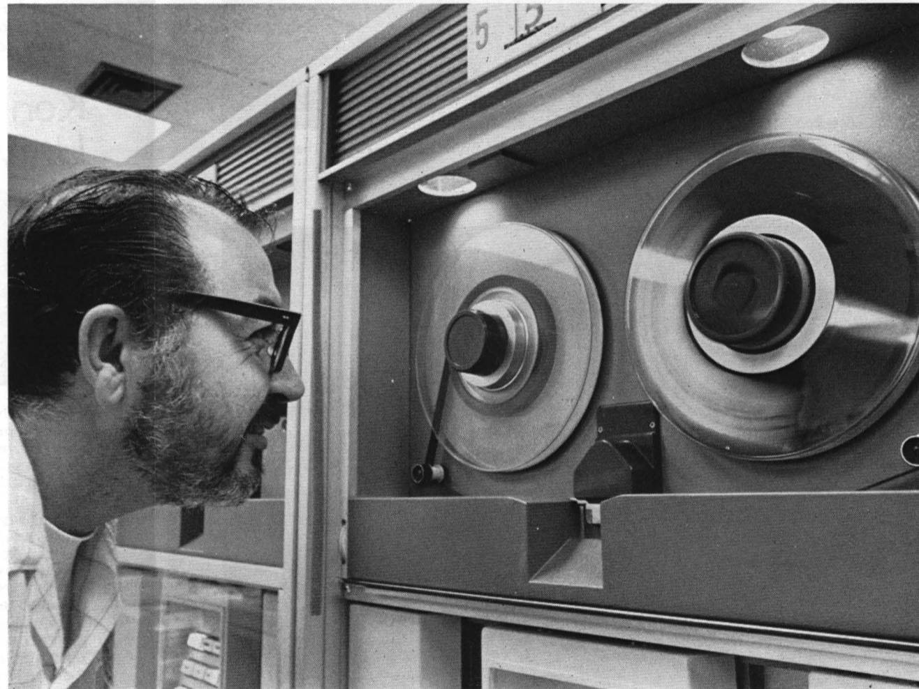
WILFRED OTERO (9411) awaits a tape being rewound. The tape is reeled at a rate of 400 inches per second.
