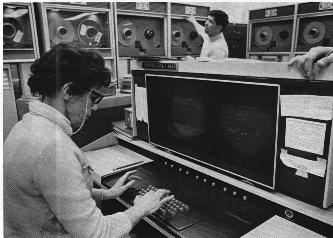
COMPUTER OPERATOR Mary Couch (9411) assigns tape to an executing program. Requests for tape appears on console screen.
