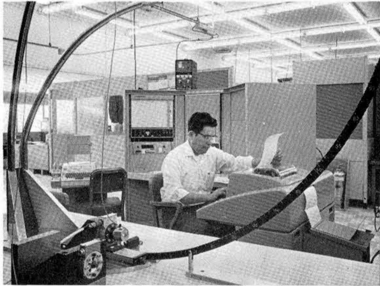
DATA OUTPUT from an automated transducer evaluation is read by Felix Almaraz. The HP 2116-B computer will eventually be connected to most test equipment in the Menaul Facility. In foreground is a ballistic pendulum used to calibrate shock accelerometers.
