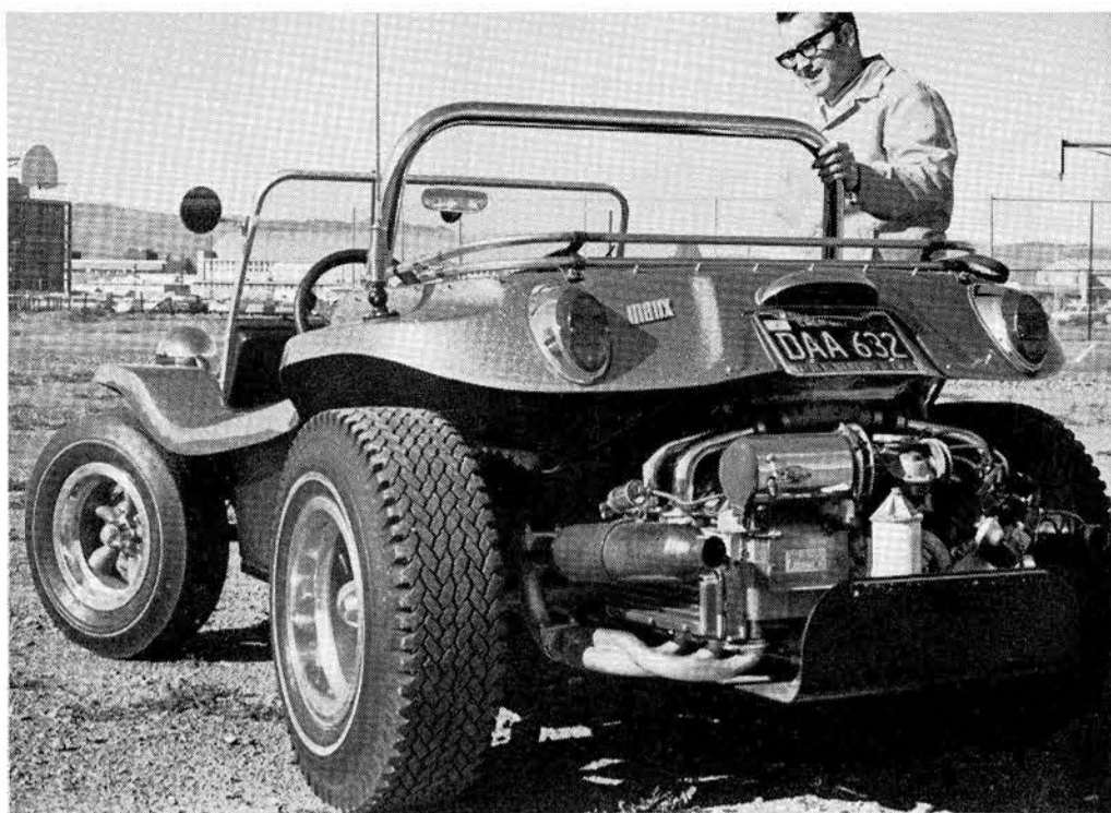
170-HORSEPOWER ENGINE is unique feature of Manx dune buggy built by Jerry Henderson (8162) in his spare time. Polished "mag" wheels and a $700 fiberglass body add to class as well as cost.
