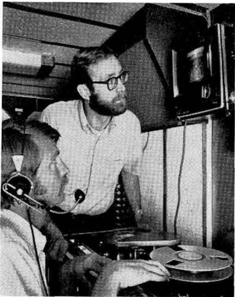
REAL-TIME RECORDS of the formation of stress patterns are made with the aid of videotape. As the cylinder is stressed it is viewed by a TV camera through an earlier hologram made of the cylinder in a non-stressed state. This produces the fringe patterns characteristic of the double-exposed still photos—but on a real-time basis. Here Carl Murphy (7362) watches the TV monitor with videotape operator Hugh Taylor (3454).
