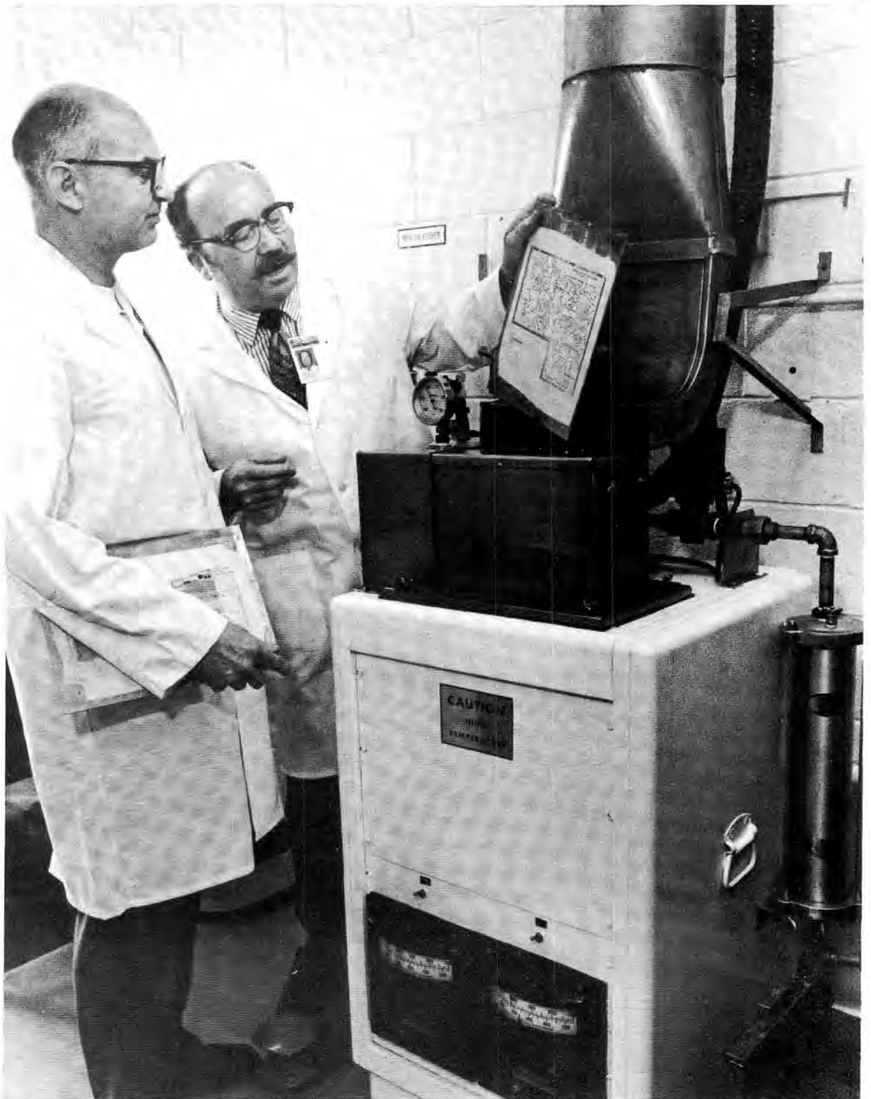
BOB SYLVESTER AND T.A. ALLEN (both 7123) examine printed circuit board emerging from machine they've developed that levels solder on PCB with blast of hot air.
