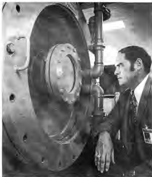
GEORGE WRIGHT (5628) heads ASTM committee which recently completed work on a new standard for testing for heat of ablation. One of the tools used in the work was the HEAT facility in Area III which produces a jet of high energy gas to simulate heat of reentry.
