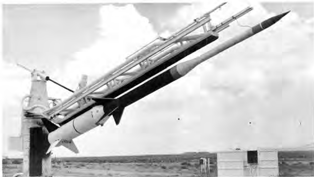
TATER, three-stage rocket system developed by Sandia, achieved a velocity of 10,700 feet per second in the heavy atmosphere under 11,000 feet. The successful first flight of the system was conducted recently at Tonopah Test Range.
