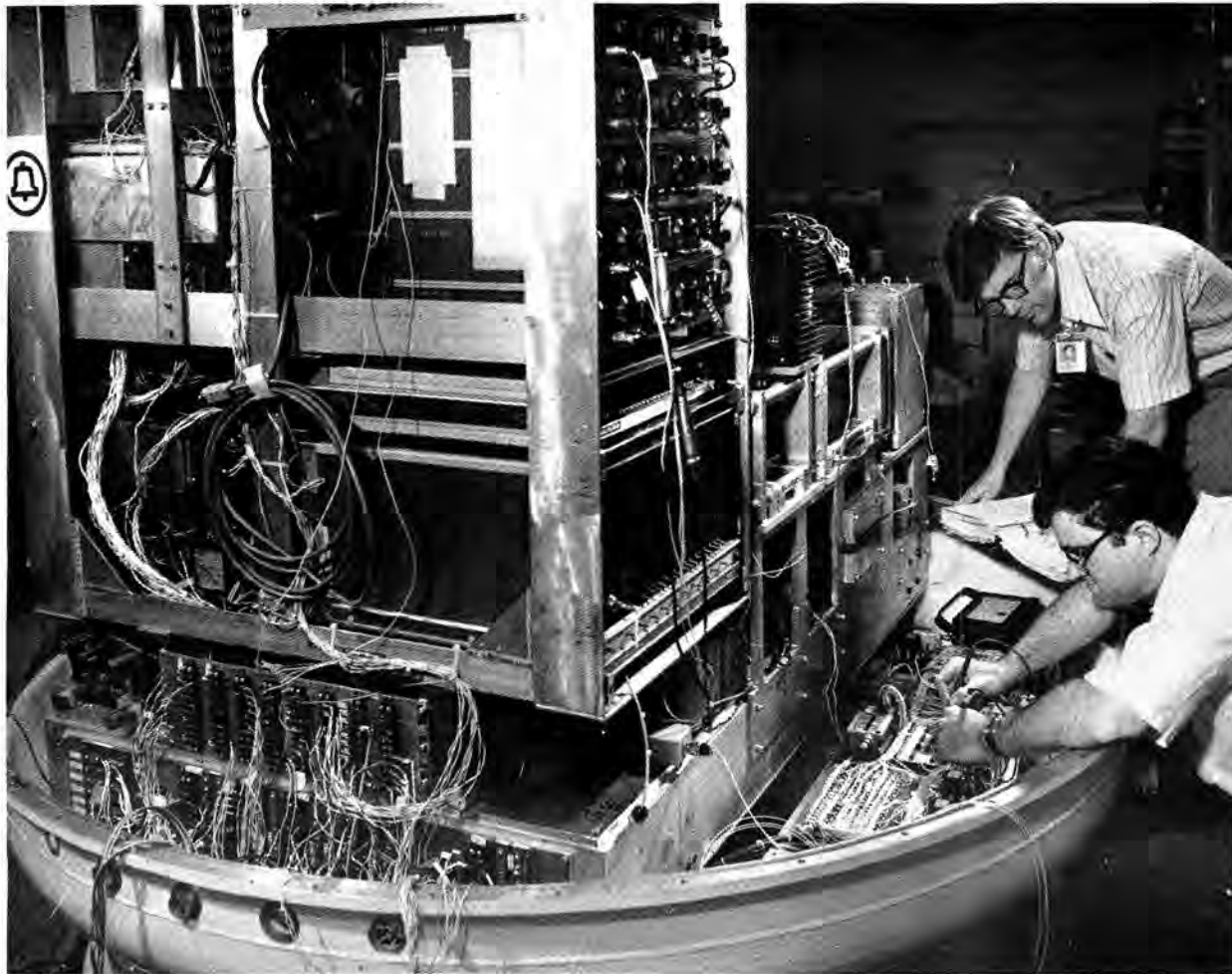
INSTRUMENTATION PACKAGE for the balloon flight May 15 is readied in Bldg. 892 High Bay area. Here, project leader Al Watts (1255), and BTL engineer Gardner Burkhardt work on the 5000-lb. payload.
