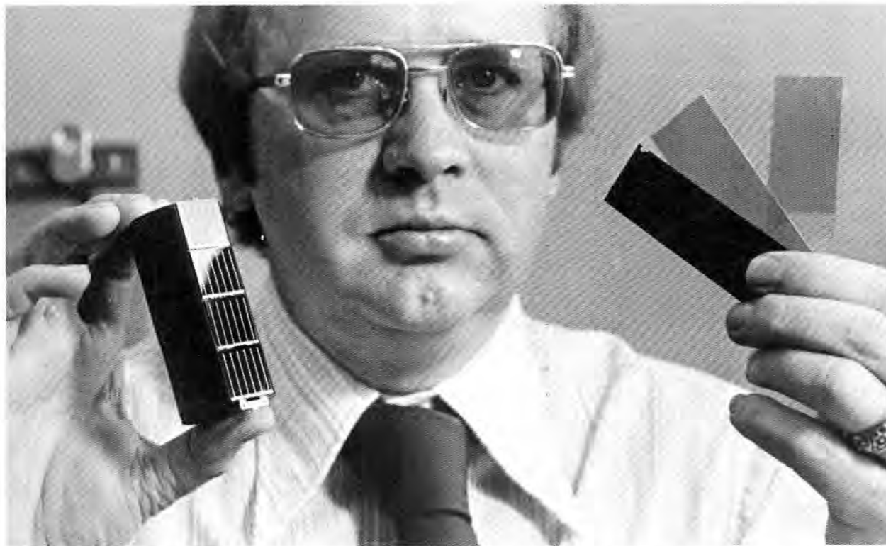
A DECK of four solar cells (left), for direct conversion of solar energy to electricity, is mounted upon a thermal collector pipe which converts solar energy to heat. Right, samples of thin films which may supersede silicon as the working material of solar cells. Don Schueler (5113) heads the Photovoltaic Working Group.
