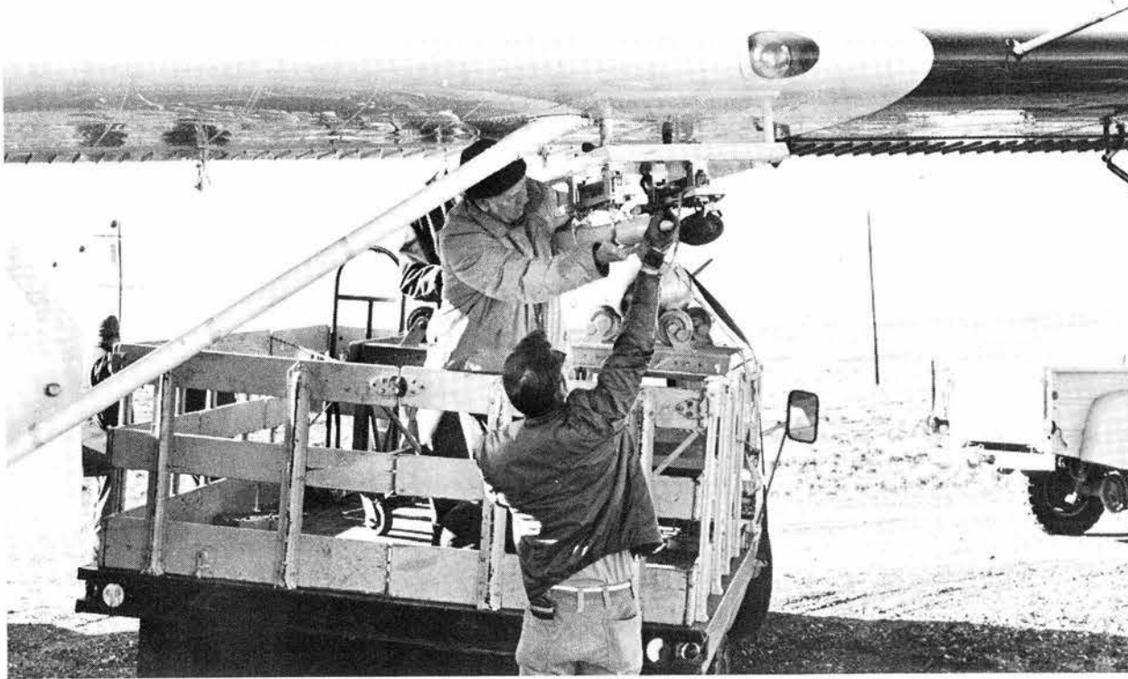
LEO DUNN (9414) and CHARLIE MONROE (9754) load ice penetrator unit onto wing rack of Sandia's Beaver aircraft for drop testing at Edgewood Test Range. Three units were dropped from 6000 ft. altitude into the frozen earth target at the range. Wayne Young (5716), project leader, reports the tests were successful. Sixteen units, which measure sea ice thickness, temperature, and other characteristics, will be dropped in April north of Point Barrow, Alaska, for the U.S. Navy. The Sandians will operate out of the Naval Arctic Research Laboratories in Point Barrow.
