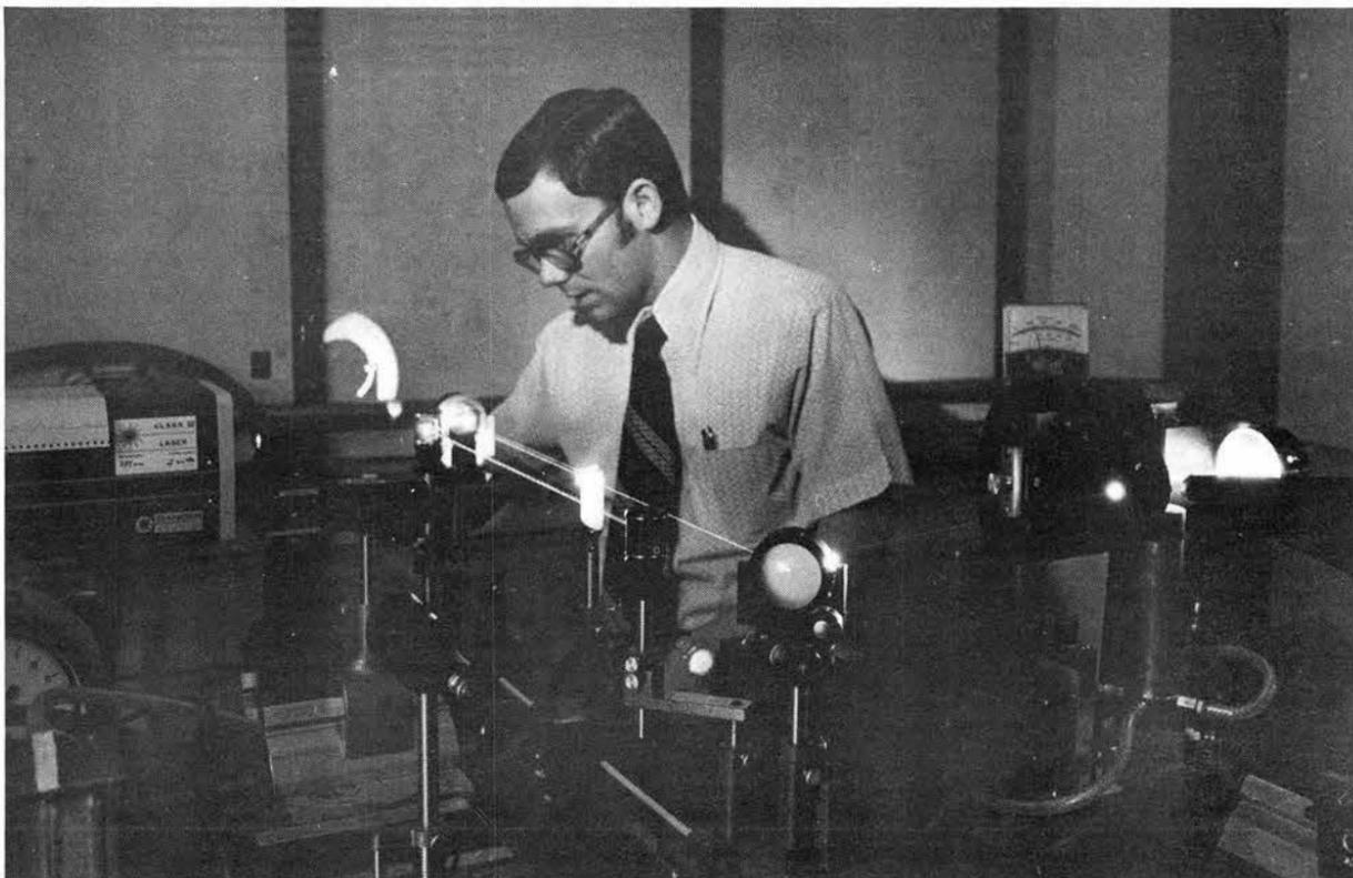
RAMAN SCATTERING is used for measuring species concentrations and temperatures in both laminar and turbulent flames during reacting flow studies. Bob Setchell (8115) adjusts laser for the laminar experiment.
