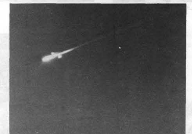
HEAT SHIELDS on side of rocket pop out to slow vehicle for recovery. Photos (including F-4J on page one) were taken with Sandia's 596.9 centimetre focal length LA-24 tracking telescope at a distance of more than 50 Kilometres (30 miles) on 70mm film.
