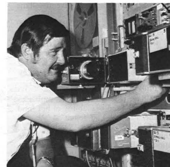
JOHN BROUILLARD (1131) readies equipment for measuring ground shock very close to the nuclear device for an upcoming LASL underground event.
