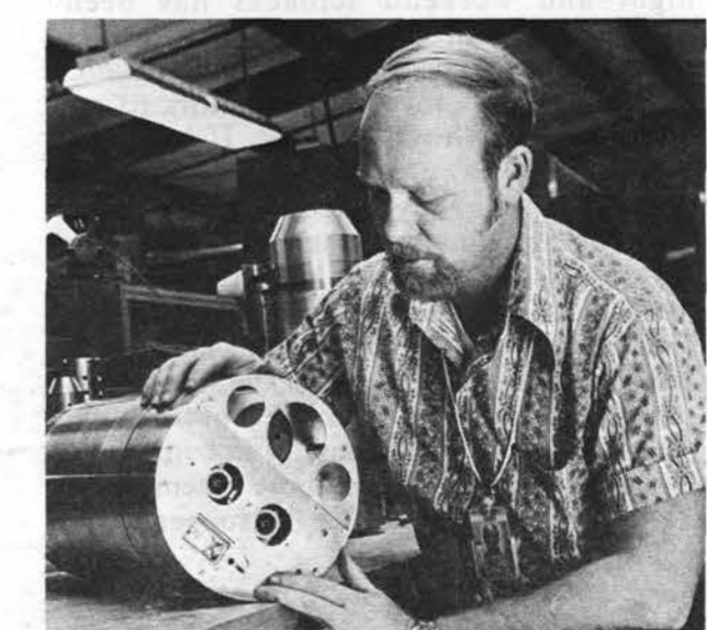
DON SHADEL (1131) readies a downhole television camera. Unit has built-in light source and wide angle lens.
