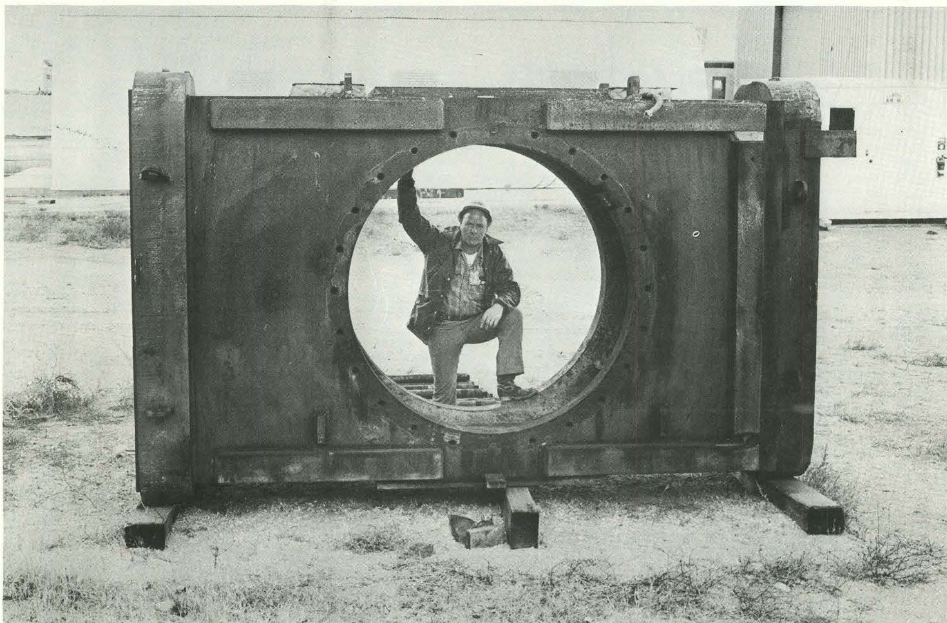
BILL BLYTHE (1131), one of Sandia's engineering and construction coordinators at Nevada Test Site, is shown with one of the giant closure gates used in underground testing. Massive steel doors, powered by compressed gas, close within 16 milliseconds after firing, allow passage of initial burst of
