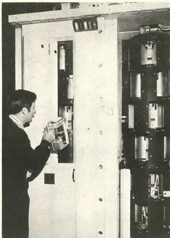
DUANE ARLOWE demonstrates method of placing a canister, which holds up to 2½ kilograms of SNM, in a carousel. Carousels and canisters are part of an advanced storage vault and protection system being developed by Sandia for ERDA's Division of Safeguards and Security.
