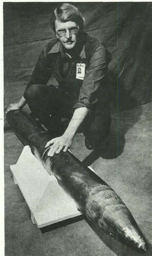
GENE HARTY (4342) displays prototype Pershing II earth penetrator unit recently recovered from 33 metres beneath the surface at White Sands Missile Range. A "quicksand" earth formation hampered recovery efforts. The unit was finally removed after stabilizing the surrounding material by freezing it with liquid nitrogen.
