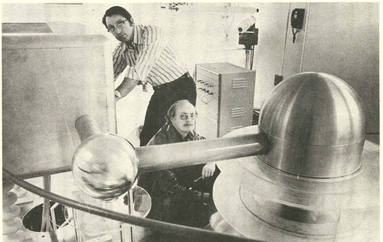
NEW 250 kV deuterium ion accelerator is complete and installed in an underground laboratory in Bldg. 807. Division 2354 will use the new machine to bombard scandium and erbium hydride films to create neutrons; the neutrons offer a promising new way to treat cancer victims. The program, financed at $500,000 by the National Cancer Institute, will explore the upper limits of neutron production using solid target neutron generators. Ultimate aim of the program is to develop design parameters for a clinically useful machine. Preparing the new accelerator for gradually increasing power output tests are Al Riedel (2354), standing, and Frank Bacon (2354), project engineer.
