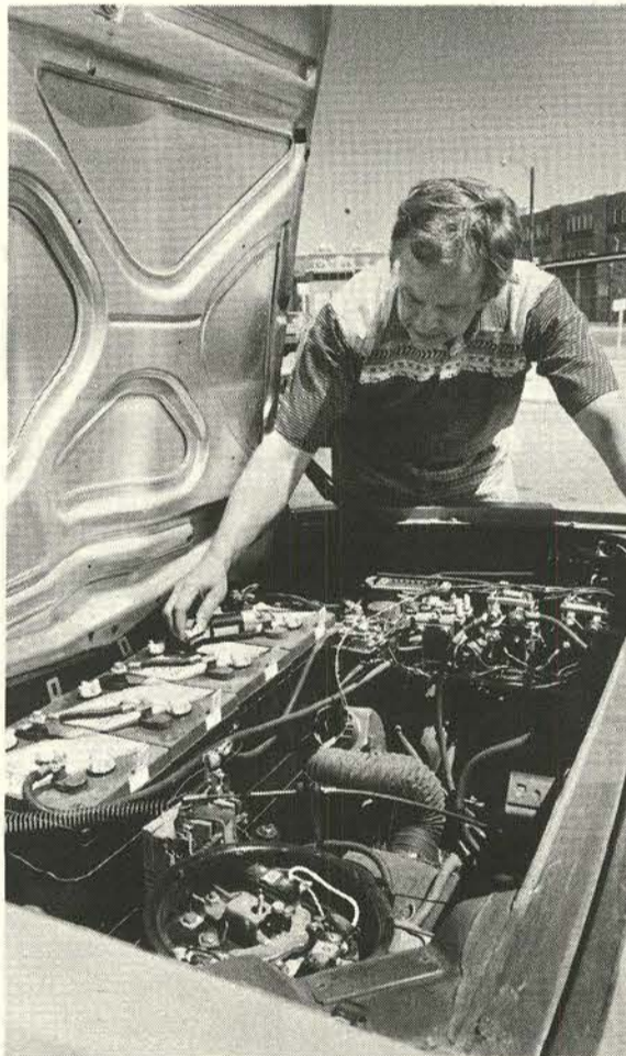
DICK BASSETT'S NEWEST ELECTRIC CAR allows him to commute from the far North Valley to Sandia. And back. Below, Dick fingers a fuse which permits temporary overloading of system for brief bursts of power.
