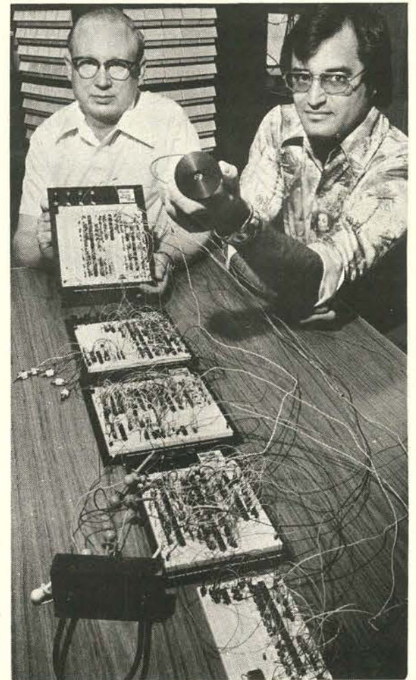
SOPHISTICATED SEAL is held by John Aragon (1754), right. The breadboard version of the new seal's electronics, which require over 80 integrated circuits is displayed by Larry Hermesmeier (1754). Sandia is incorporating these functions into a single integrated circuit and a small package that cannot be opened without detection. Any tampering with the fiber optic loop causes a change in the sequence of code symbols visible in the seal's window (here an 8).
