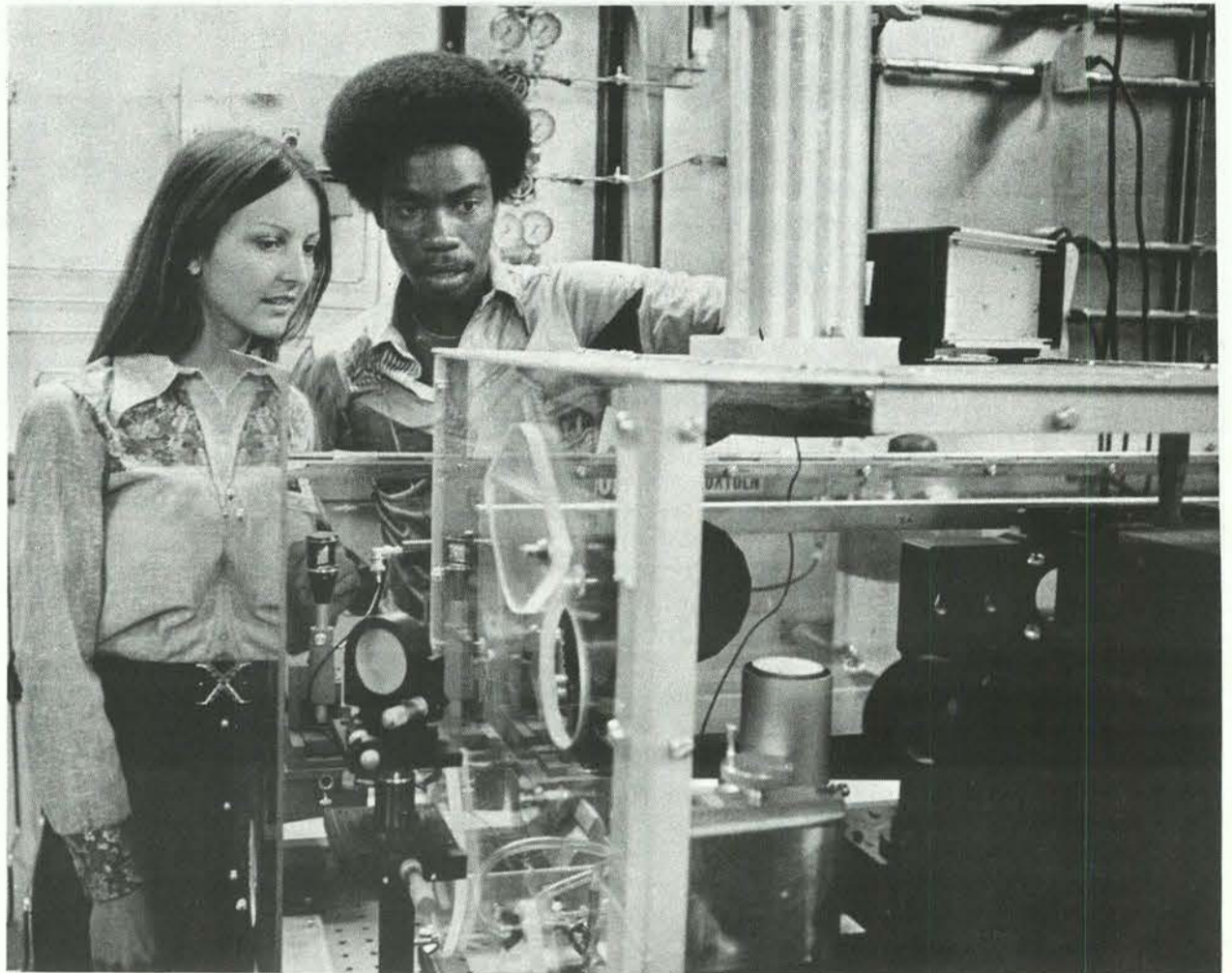
SUZI SCHOENUNG, Sandia summer hire, and Reggie Mitchell (8351) have spent the last three months making some of the most sensitive temperature measurements taken to date at Sandia. They used the laser Raman spectroscopy setup in SLL's ambient-pressure flame facility. Suzi returns to Stanford this fall.
