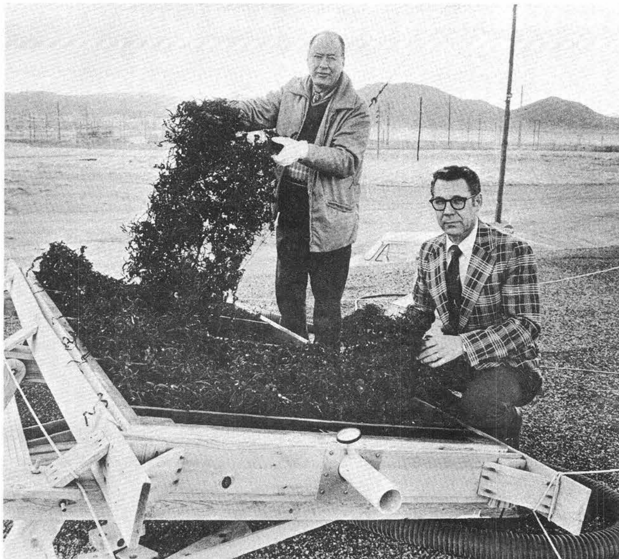
RAY BRIN (9410) AND TOM PACE (9420) display blackened aluminum lathe turnings which greatly enhance heat absorption in their newly-patented flat-plate solar energy collector. Glass pane covers the collector box when in use.
