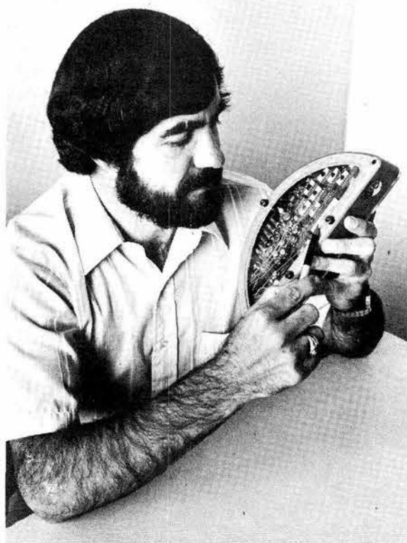
JIM CARUTHERS (2332) points out the microprocessor (the small square) which is the heart of the MC3152 programmer. The component fills one-half the volume, is one-fourth the weight of its predecessor, and costs half as much.
