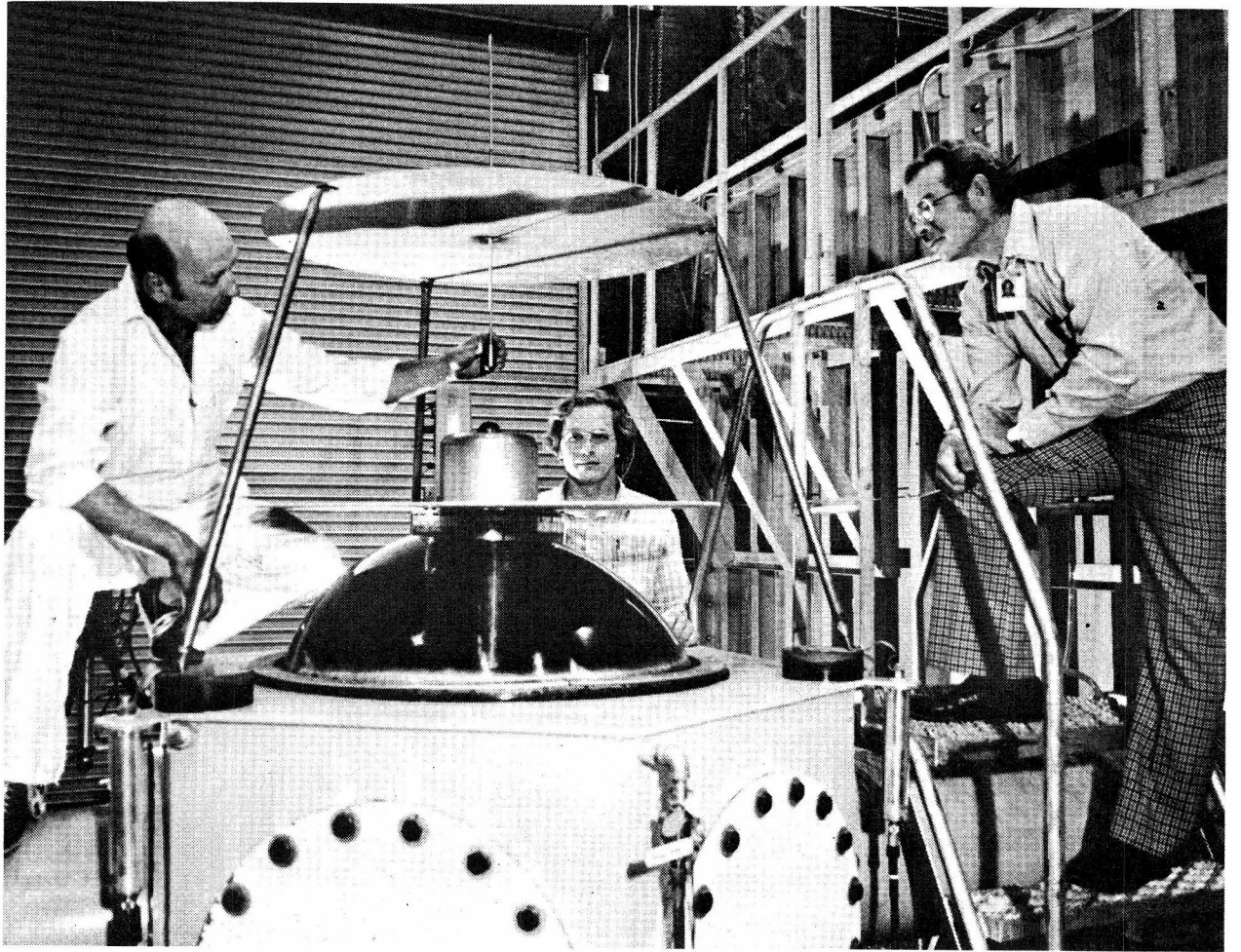
AT THE lightning simulator facility, Bill Brigham makes an adjustment to the load ring (the name of the entire apparatus), while Joe Kostas (center) and Jim Bushnell (all 1554) look on. At right foreground is one of the two oil-filled tanks housing Marx generators which generate the simulated lightning charge. The charge rises through the black plexiglass dome (which is filled with oil for insulation). The current is conducted to the top of the electrode where it arcs up to zap a test component which would be suspended above the load ring.
