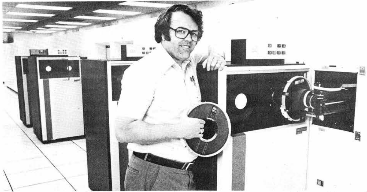
THE NEW Integrated File Store provides central storage for user programs and data, and is accessible from any Sandia computer. Bill Huntman (2645), who designed the facility, stands next to the 96-foot-long magnetic tape cabinet.
