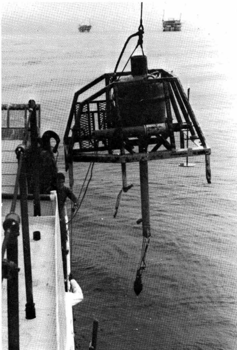
OFF THE SEAFLOOR comes a SEMS device after a year of collecting seismic data in the Santa Barbara Channel. Units provided new insight into seafloor behavior.
