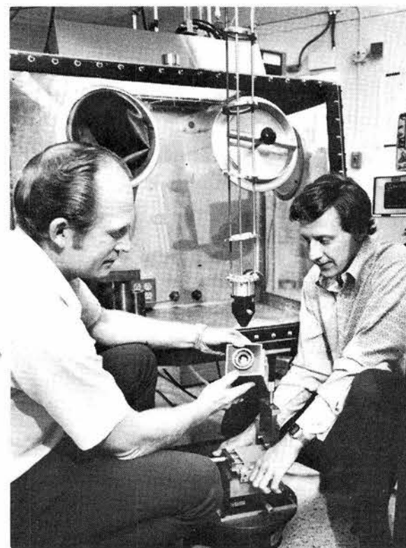
DISPLAYING a sensor containing 10,000 photo-diodes are Larry Pope, left, and Tom McDonald (both 5833). The sensor is a component in the laser diagnostic tester, developed by them, which will improve welding techniques used in the assembly of critical components.
