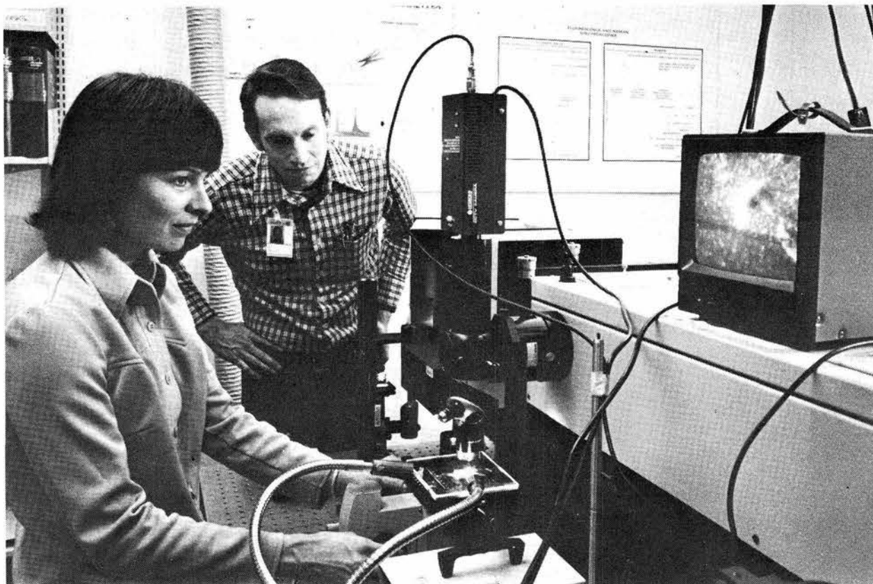
OBSERVING an epoxy particle magnified 100 times are Karen Higgins and Dave Tallant (both 5823). Karen is operating the laser fluorescence/Raman microanalyzer which displays magnified images on the TV screen. The microanalyzer, which uses continuous and pulsed laser beams in conjunction with a microscope, provides quick and accurate chemical identification of small particles.
