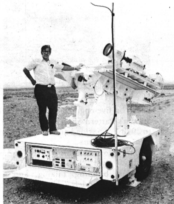
BOB SCHOWERS (7171) displays new tracking camera with lightweight mount, 60-inch telescope, and TV camera. The new unit is easily moved, can be positioned at any point on the range to provide additional coverage of air drops. The unit's minicomputer has RF link to the range's Operations Center for target acquisition.
