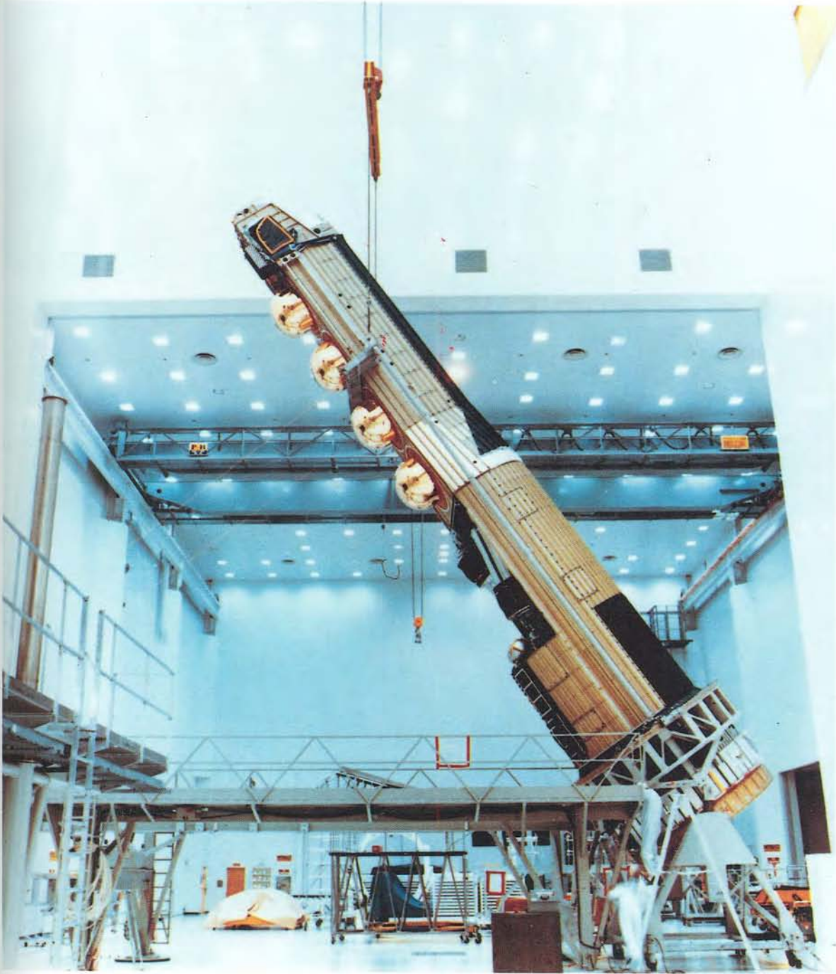
Satellite Vehicle Assembly Going Vertical
