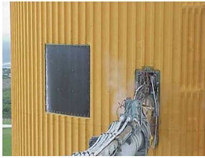
Gaseous hydrogen vent line leak caused STS-119 scrub in March 2009, also caused two scrubs on STS-127. This line connects the Ground Umbilical Carrier Plate (GUCP), attached to ET, to "flare stack" for burn-off of vented gaseous hydrogen.
