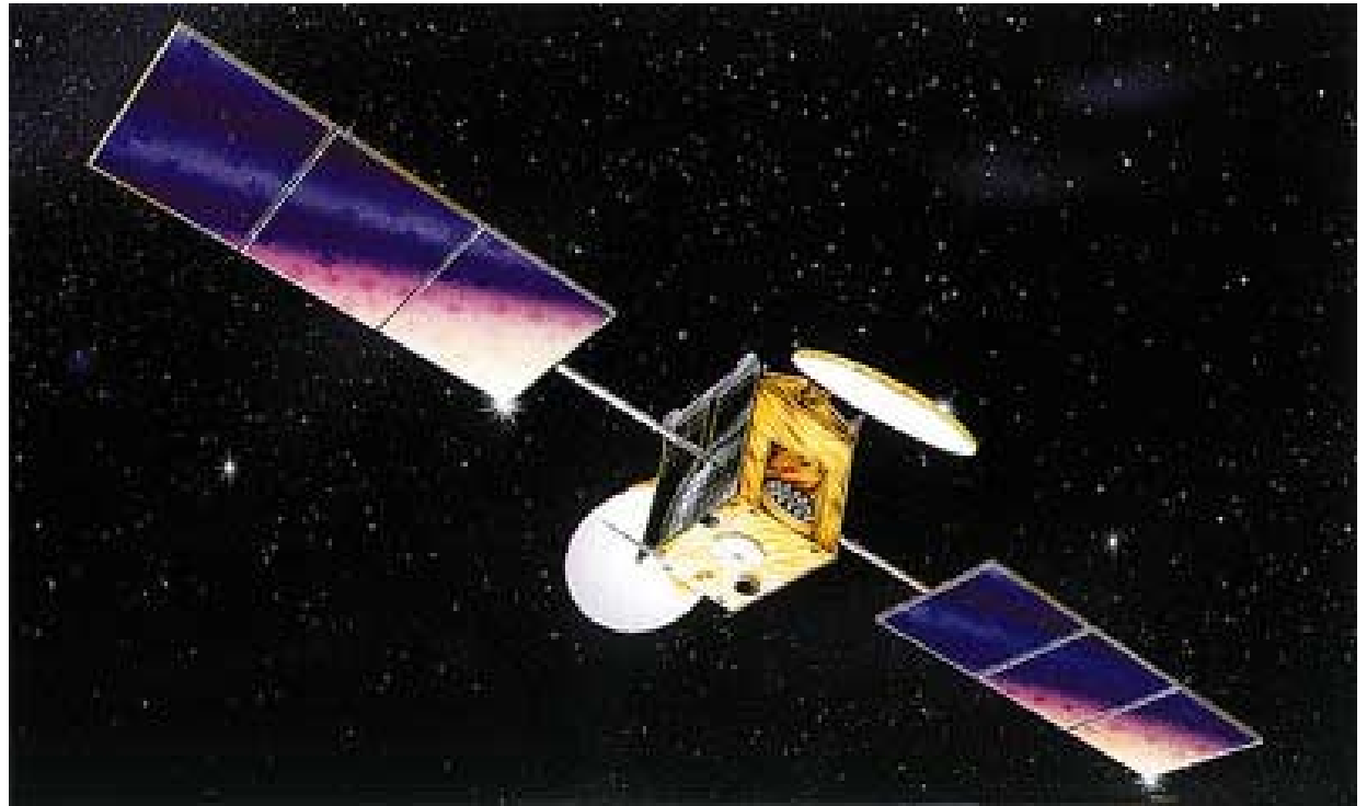
US-built INMARSAT 3 F1 satellite L-band communications payload (MMS-UK) Launched from Cape Canaveral, Apr 1996 Stationed over Indian Ocean at 64 E, May 1996
