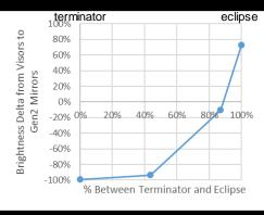
Mirrors brighter right at eclipse as near specular scatter goes to earth
