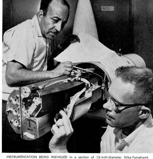
INSTRUMENTATION BEING INSTALLED in a section of 12-inch-diameter Nike-Tomahawk by Adolfo Martinez (left) and D. R. Kuehl (both 9221) will be used to measure the density of molecular oxygen by observing the absorption of solar radiation.
