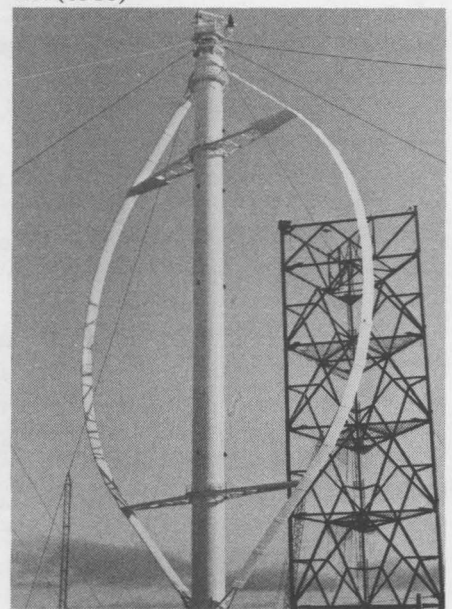
EOLE, a 110-m (360-ft.) vertical axis wind turbine in Quebec, Canada, includes Sandia-designed features.
