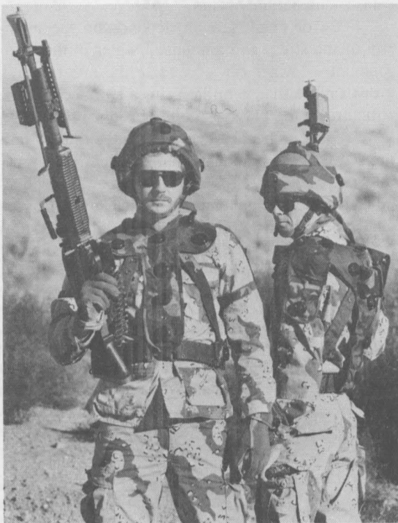
JIM KAISER (left) and Jeff Johnson (both 3435) provide a close-up look at the front and back of the TESS detector vest. The vest's detectors, strategically placed in a T-arrangement, accurately record close-in "kills" during counter-terrorist training exercises. Small rectangular packages near the barrel end of Jim's M-60 and Jeff's M-16 are TESS laser transmitters.
